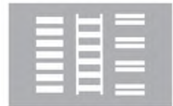
Typical crosswalk markings: Continental, Ladder, and Staggered Continental (Credit: Michele Weisbart)
