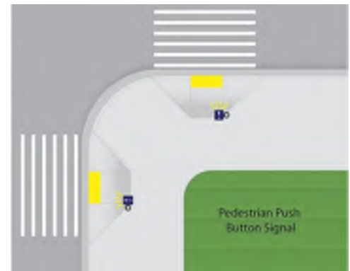
Pedestrian push button placement (Credit: Michele Weisbart)
