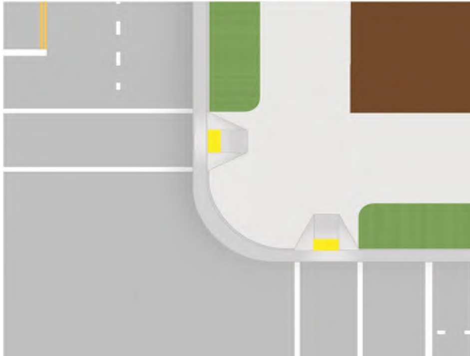
One curb ramp per crosswalk should be provided at corners. Ramps should align with sidewalks and crosswalks. (Credit: Michele Weisbart)
