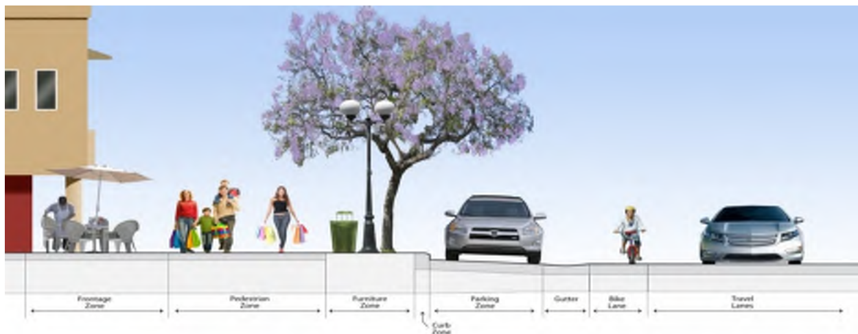
An example of integrating curb extensions and parking into the sidewalk corridor by placing a valley gutter between the parking and the traveled way. (Credit: Michele Weisbart)
